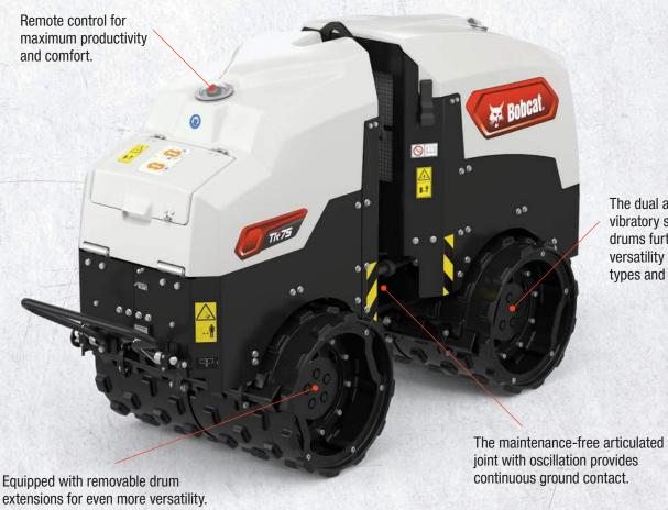
The dual amplitude vibratory system in the drums further enhances versatility in unique soil types and materials.
